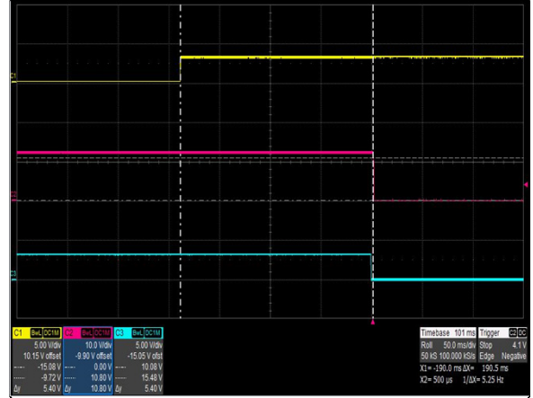
Figure 8: CSV1300BP-3 Turn Off Characteristic via PSKill Load: I_O = 106.6A I_{SB} = 2.5A Ch 1: PSKill Ch 2: V_O Ch 3: PWOK
