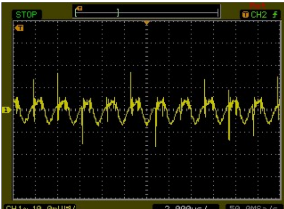
Figure 103: AXA00B36-L Ripple and Noise Measurement Vin = 48Vdc Load: Io = 0.83A Ch 1: Vo
