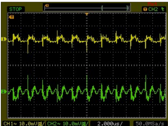
Figure 63: AXA000BB18-L Ripple and Noise Measurement Vin = 24Vdc Load: Io = ±0.41 A Ch 1: Vo1 Ch 2: Vo2
