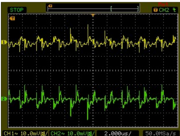
Figure 73: AXA000CC18-L Ripple and Noise Measurement Vin = 24Vdc Load: Io = ±0.33 A Ch 1: Vo1 Ch 2: Vo2
