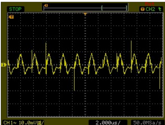
Figure 113 : AXA00C36-L Ripple and Noise Measurement Vin = 48Vdc Load: Io = 0.67A Ch 1: Vo
