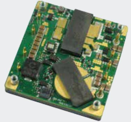
Advanced Energy's Artesyn AVE600 series half-brick isolated DC-DC converter provides a single regulated low noise 12 Vdc output that can deliver up to 50 amps. It has a wide 2:1 input range of 36 to 75 Vdc and is designed primarily for use with standard 48 V telecommunications equipment supplies. This converter is normally used in designs with a distributed power architecture (DPA), where one or more downstream non-isolated DC-DC converters meet the needs of lower voltage semiconductor devices.
