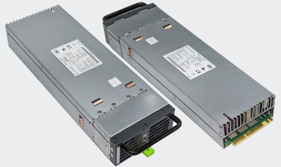
Advanced Energy's Artesyn HPS3000 series bulk front end AC-DC power supply accepts a wide range 90 to 264 VAC input and provides a main 48 V output plus a 5 V standby output. It has a full load efficiency of more than 90% and is rated at 3,000 watts when operating from a nominal 200 VAC input. Housed in a 1U x 4.2 inch form factor enclosure, the power supply has a power density of 40 watts per cubic in; four units can fit on a standard 19 in rack shelf, to provide a total of 12 kilowatts.
