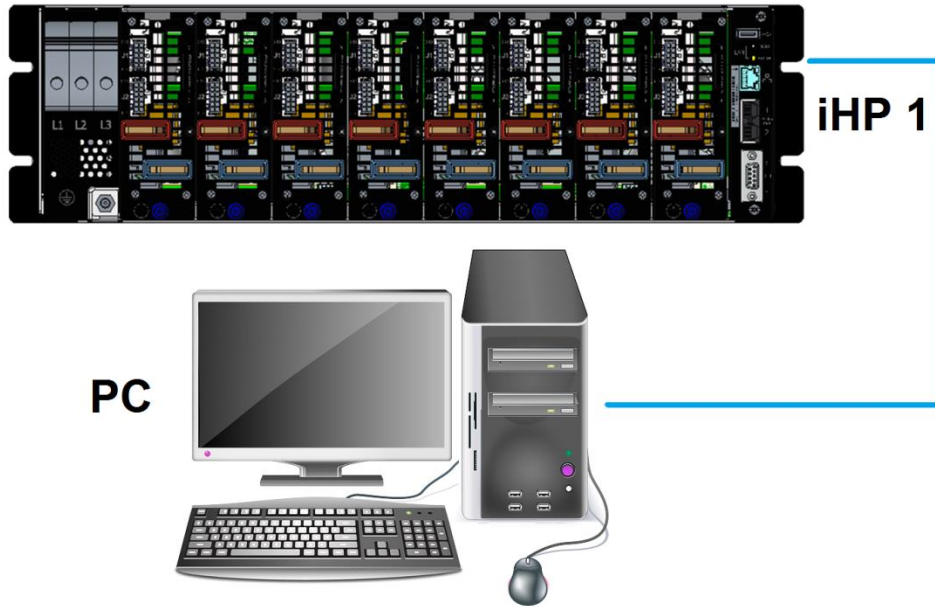
Figure 3-4 iHP system connected directly to the PC (static IP)
