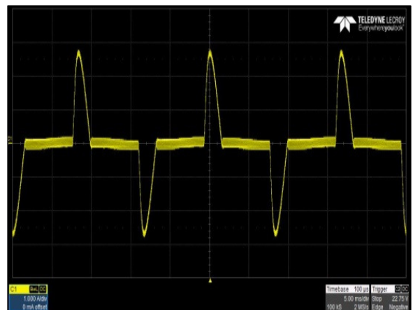
Figure 31: NPS65-M Input Current Waveform Vin = 115 Vac Load: Io = 2.5 A Ch 1: I IN
