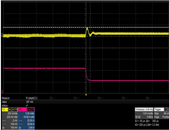
Figure 7: NPS62-M Transient Response – Vo Deviation Vin = 230 Vac Load: Io = 100% to 50%, 1 A/us slew rate Ch 1: Vo Ch 2: Io
