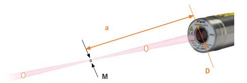
When measuring the temperature of very large and hot surfaces (for example by the float glass production), additional radiation is received by the pyrometer's detector due to unavoidable effects (diffraction, multiple reflection). These effects increase the temperature output. To get correct temperature values in this case, the pyrometer must be prepared ex works. The effect will be compensated by the float glass calibration.
