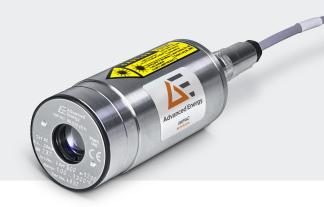
The Impac® IN 5/5 plus series infrared thermometers are specially designed for non-contact temperature measurement of glass surfaces and quartz surfaces. These instruments are digital pyrometers equipped with a digital interface, enabling temperature indication and storage on a PC. Also a temperature sub range can be configured and the instrument parameters can be adjusted remotely.
