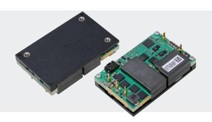
ADQ800 series quarter-brick (ADQ800-48S12B-4L) isolated DC-DC converter produces a single fully regulated 11.8 V output. Rated at 800 watts, this converter can deliver up to 70 amps output current and has no minimum load requirement. It has an input voltage range of 40 to 60 V and is primarily designed for use with standard 48 V supplies in computing and server applications, as well as regulated 48V supplies in communications equipment.
